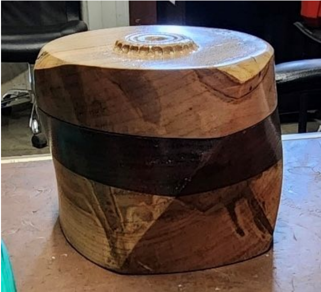
Erica Banza—Glue up of Walnut and Ambrosia Maple turned on four point axis. Finish is lacquer.
