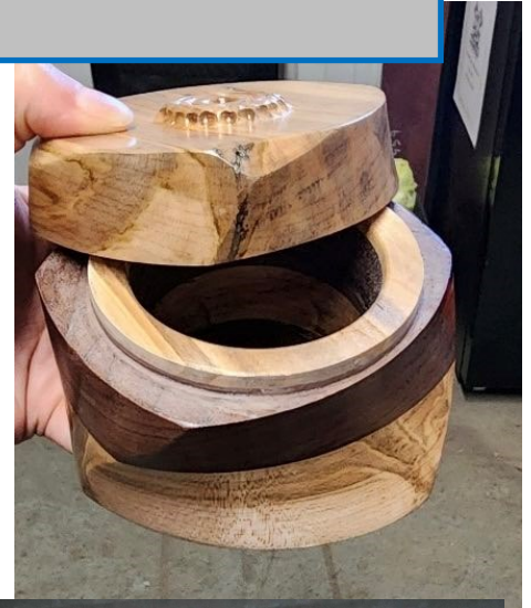
Erica Banza—Glue up of Walnut and Ambrosia Maple turned on four point axis. Finish is lacquer.
